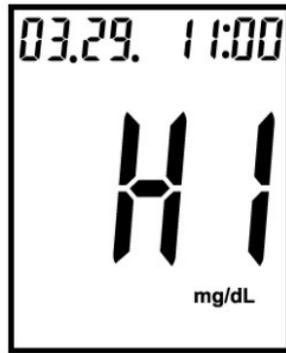
Test result is higher than 600 mg/dL.
