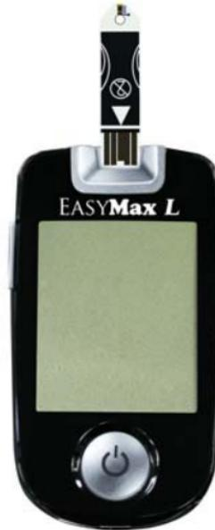
2. Put a test strip into the meter in the direction of the arrow. The meter will automatically turn on.
