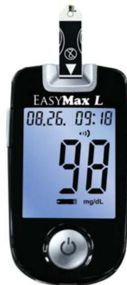
7. The meter will beep when enough blood has entered the strip's reaction zone. The result will appear on the display after 5 seconds.
